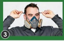
Pull the ends of the straps to adjust the tightness, beginning with the adjustment points on the head cradle and then moving to the adjustment points at the back of the neck. Do not over-tighten. Strap tension may be decreased by pushing out on back side of buckles
