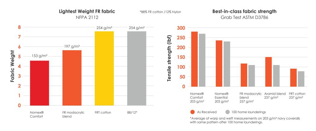
Although 100 wash cycles is the standard NFPA 2112/2113 Nomex has a test certification on 200 wash cycles independently.
